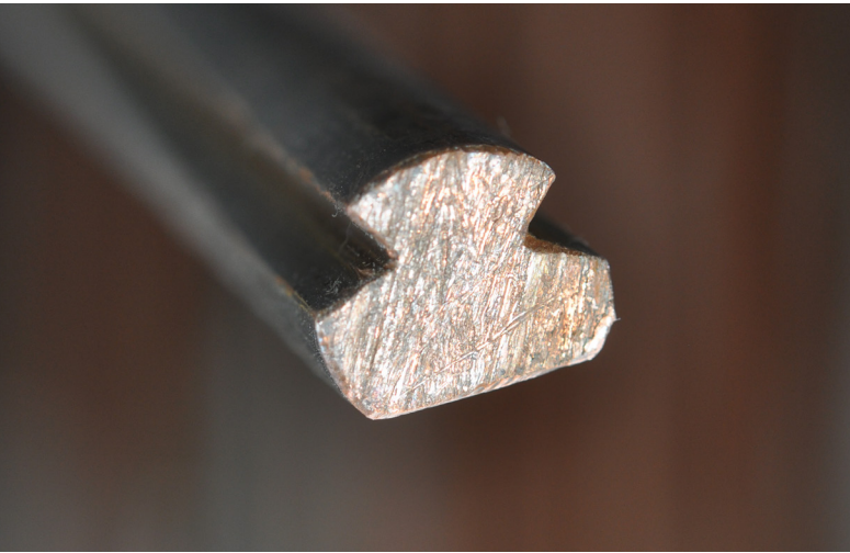
Left: Worn-out contact wires entail the risk of rupture – with severe consequences for rail traffic Right: WWS mounted on an inspection train
